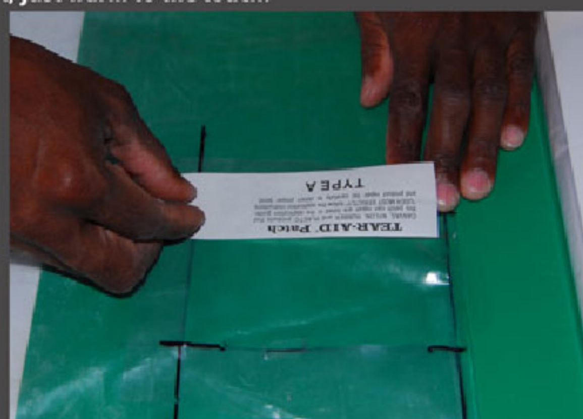
Peel back the 1 inch type A Tear-Aid tape for a cm, align the tape, stick it and peel back the tape keeping the seam of the repair in the center of the tape. The guide lines will help you with the alignment of the tape
