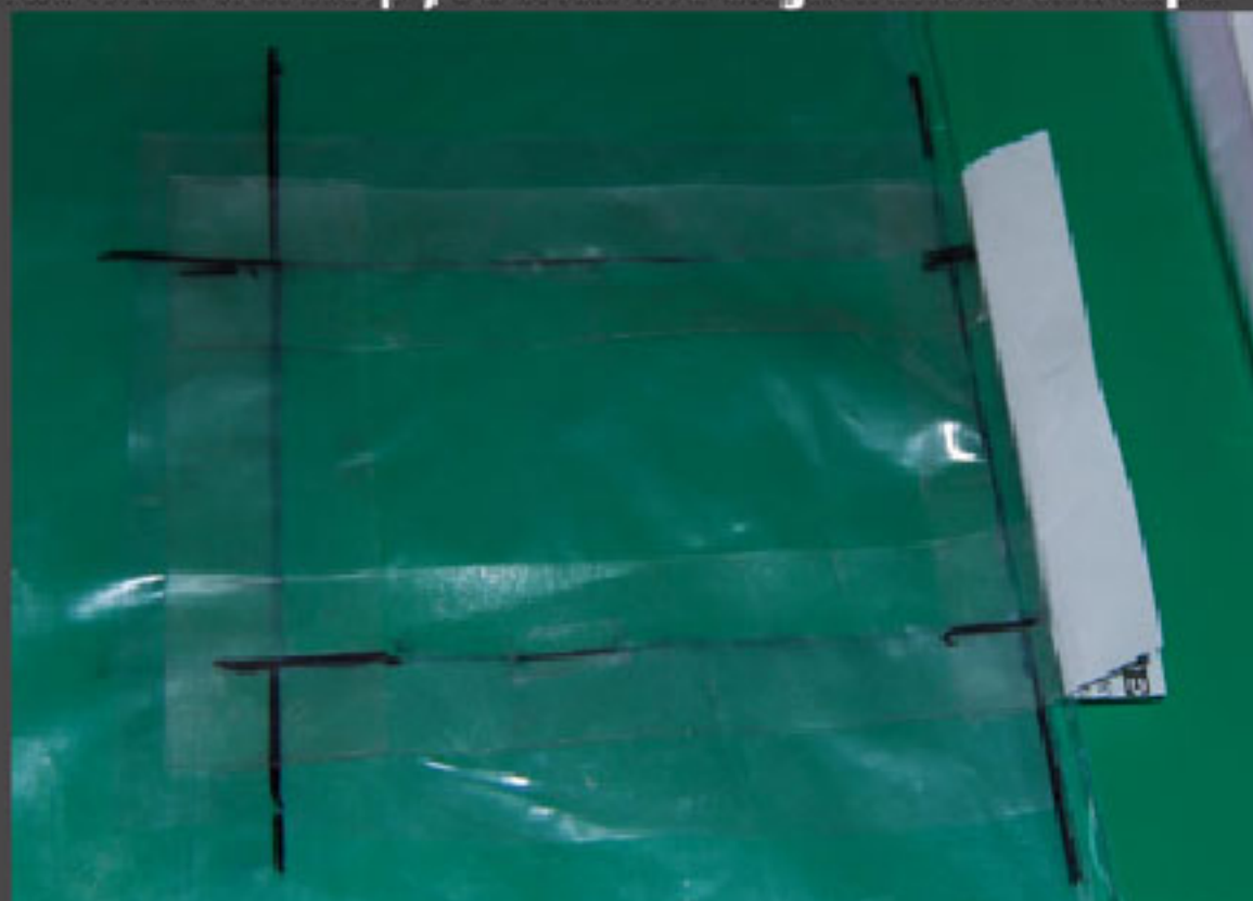
Peel back the 1 inch type A Tear-Aid tape for a cm, align the tape, stick it and peel back the tape keeping the seam of the repair in the center of the tape. The guide lines will help you with the alignment of the tape
