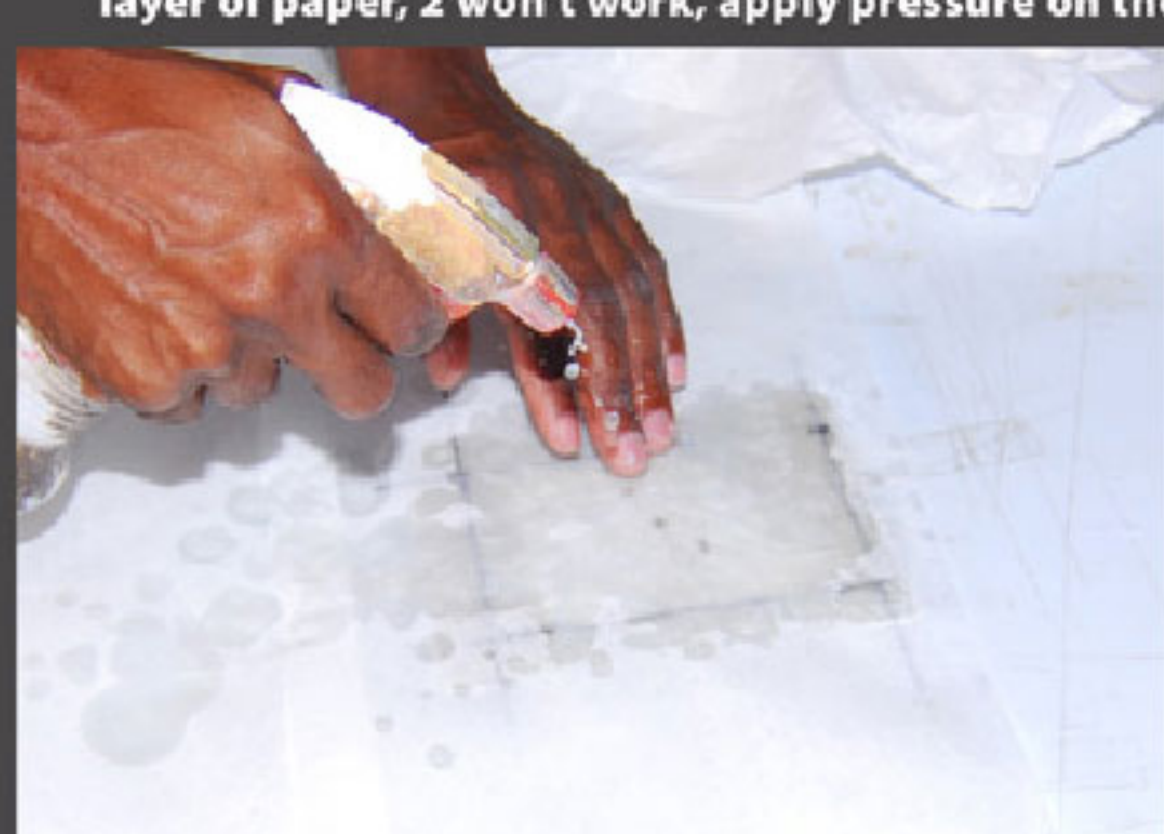
Make sure not to overheat this stage you only want to warm the glue so it flows in all the cracks and so seals the seam perfectly, to get the paper of spray on water and let the repair cool to cold before pressurizing.
