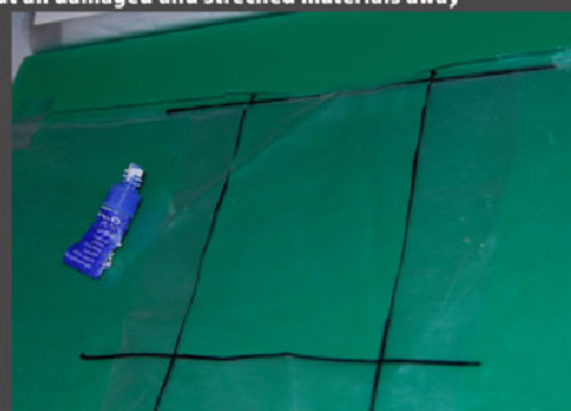
From an old bladder cut a clean piece of poly that is bigger than the marked hole, place this on the inside and secure the patch in place with little dots of crazy glue. The glue is only to keep the materials in place.
