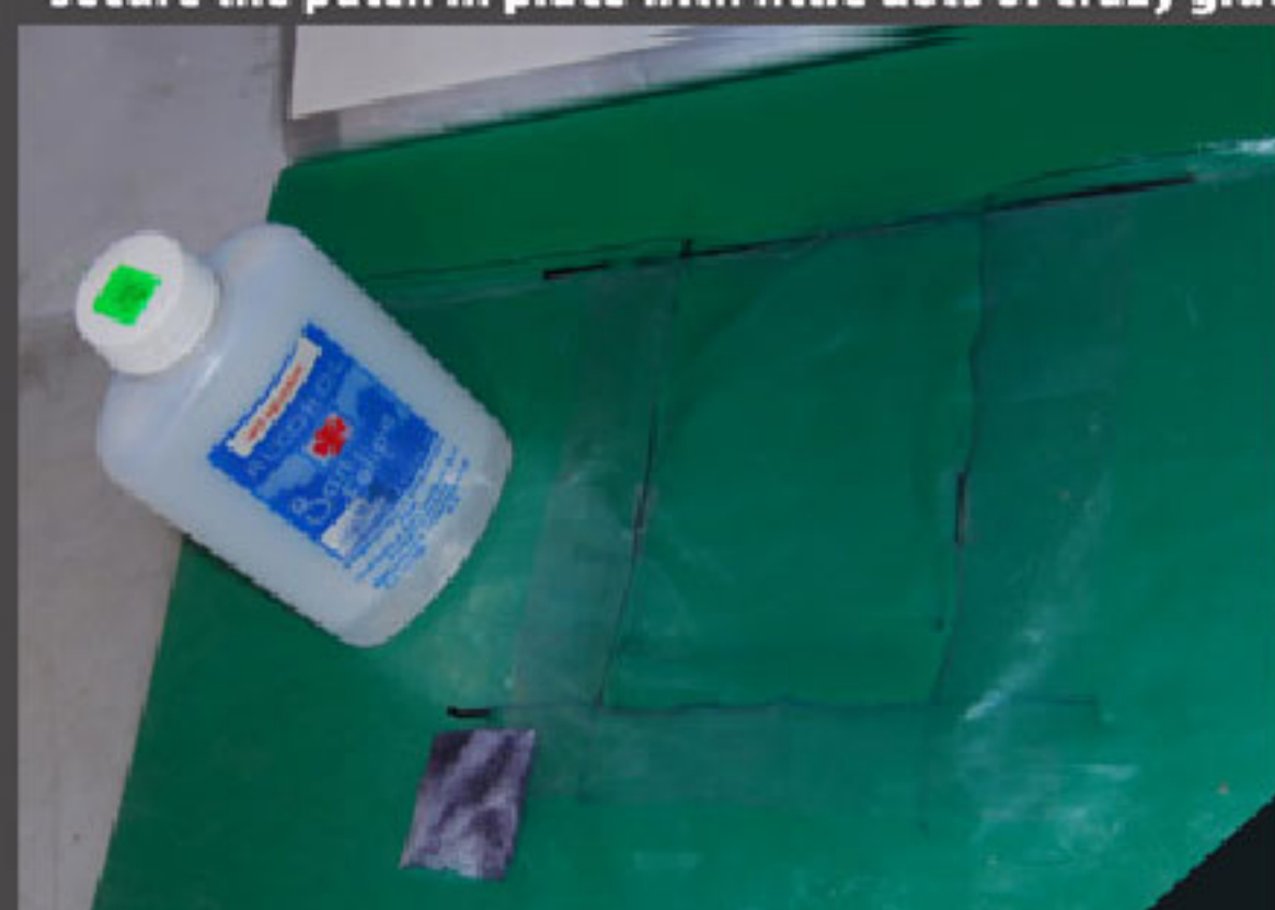
Use alcohol to clean all the surfaces then use paper towel and a warm Iron to dry out the water the alcohol left. Make sure the Iron is not hot, just warm to the touch.
