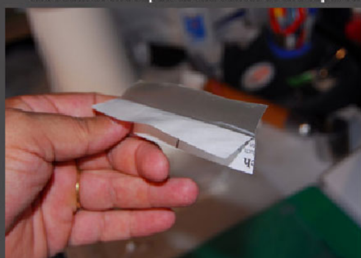
Peel back the 1 inch type A Tear-Aid tape for a cm, align the tape, stick it and peel back the tape keeping the seam of the repair in the center of the tape. The guide lines will help you with the alignment of the tape
