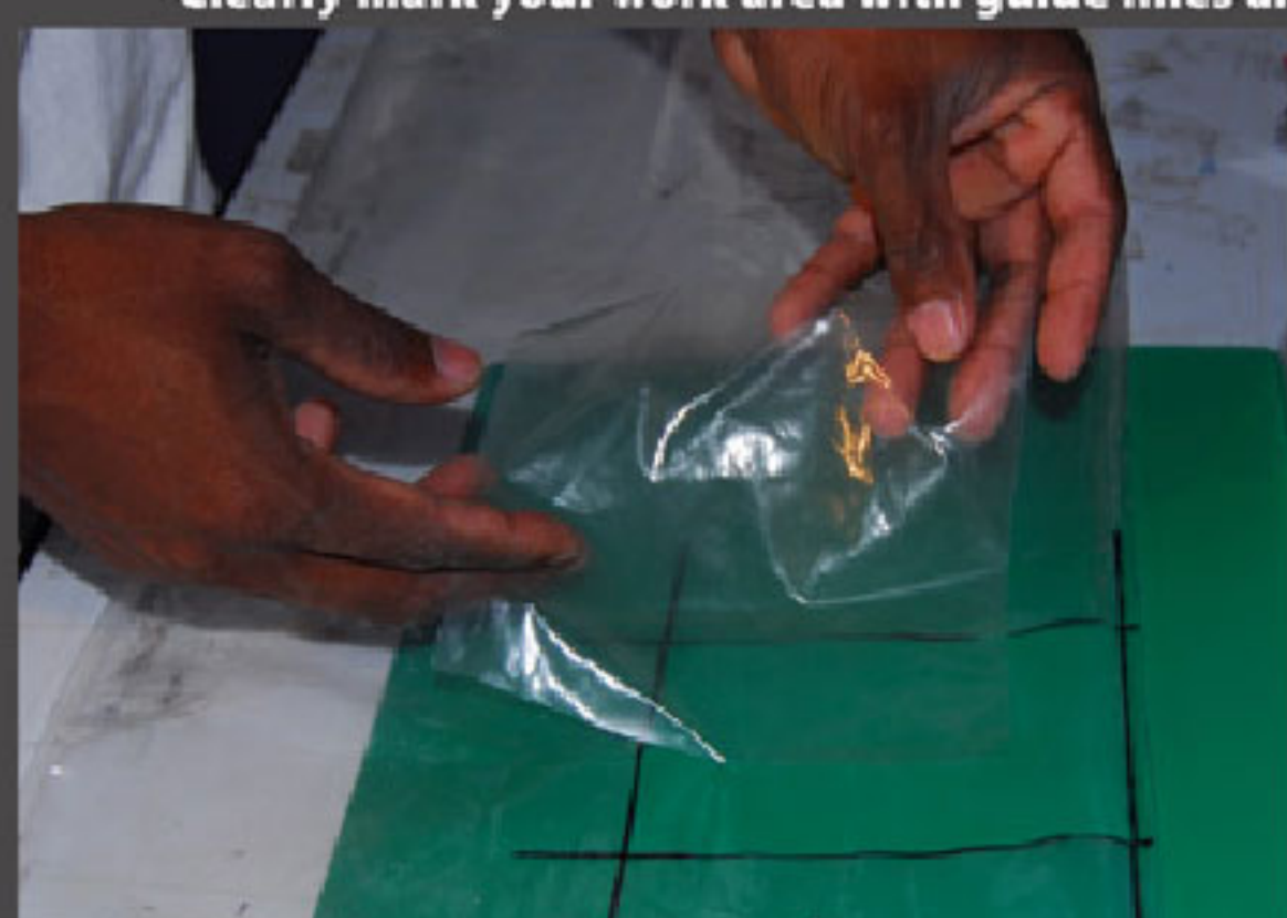
From an old bladder cut a clean piece of poly that is bigger than the marked hole, place this on the inside and secure the patch in place with little dots of crazy glue. The glue is only to keep the materials in place.
