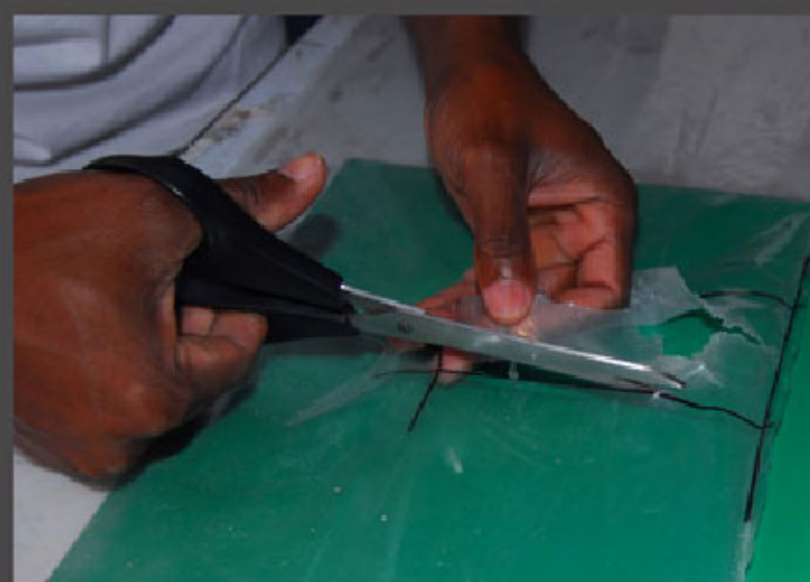
Secure the bladder with masking tape so that it will not move while you work. Clearly mark your work area with guide lines and cut all damaged and stretched materials away
