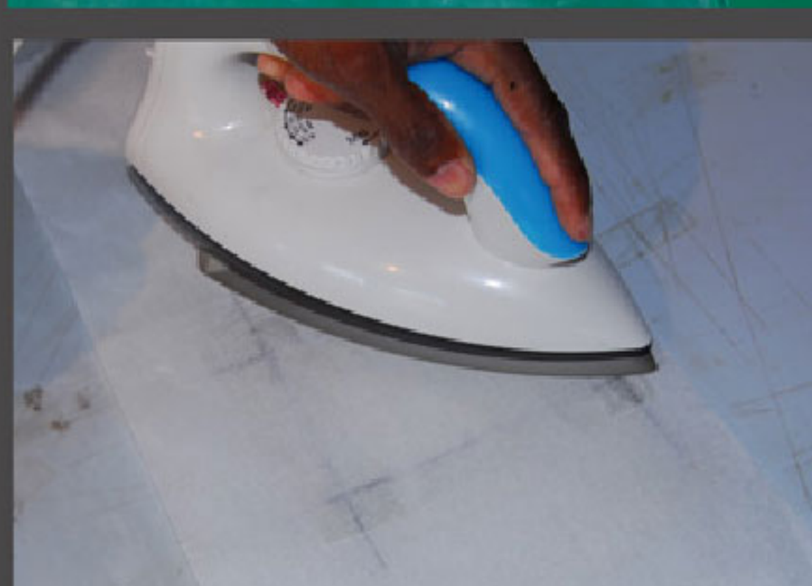
Use an Iron set to "Silk" and paper to heat up the Tear Aid tape, make sure that the bladder is covered with one layer of paper, 2 won't work, apply pressure on the iron you will see the tape bleed through the paper towel
