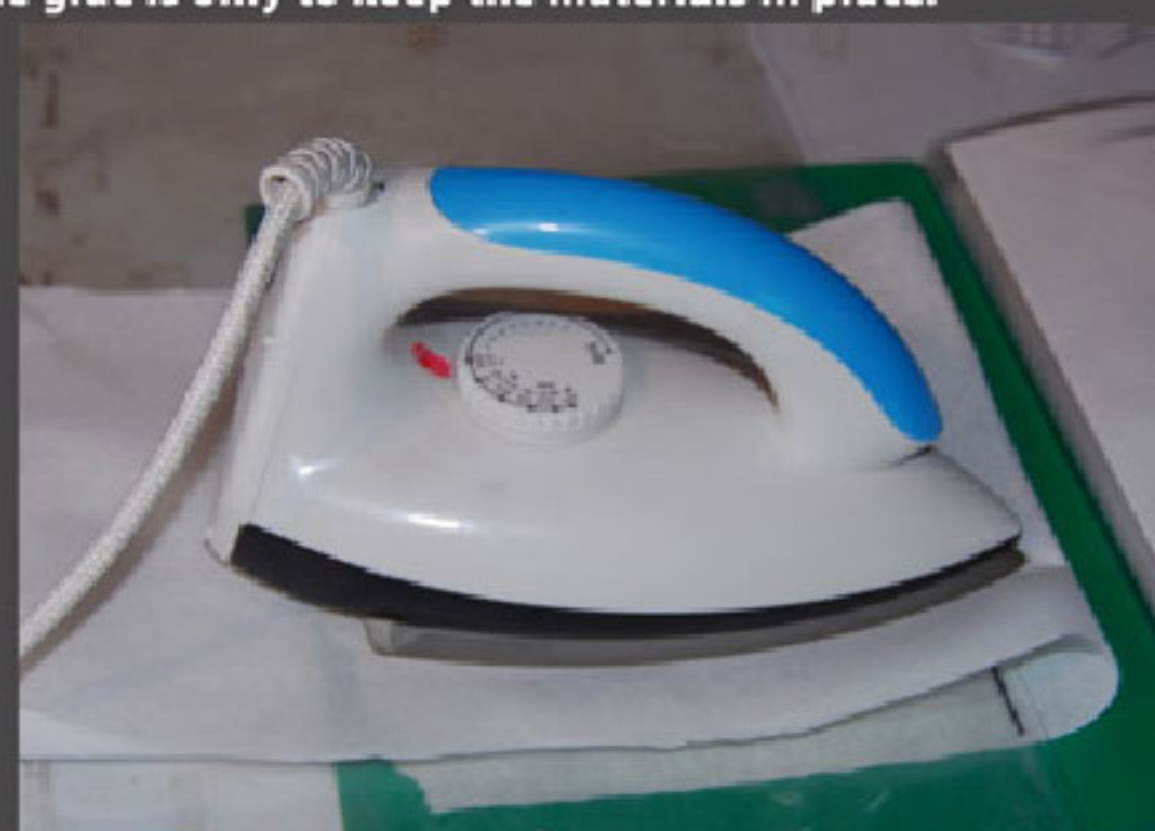
Use alcohol to clean all the surfaces then use paper towel and a warm Iron to dry out the water the alcohol left. Make sure the Iron is not hot, just warm to the touch.
